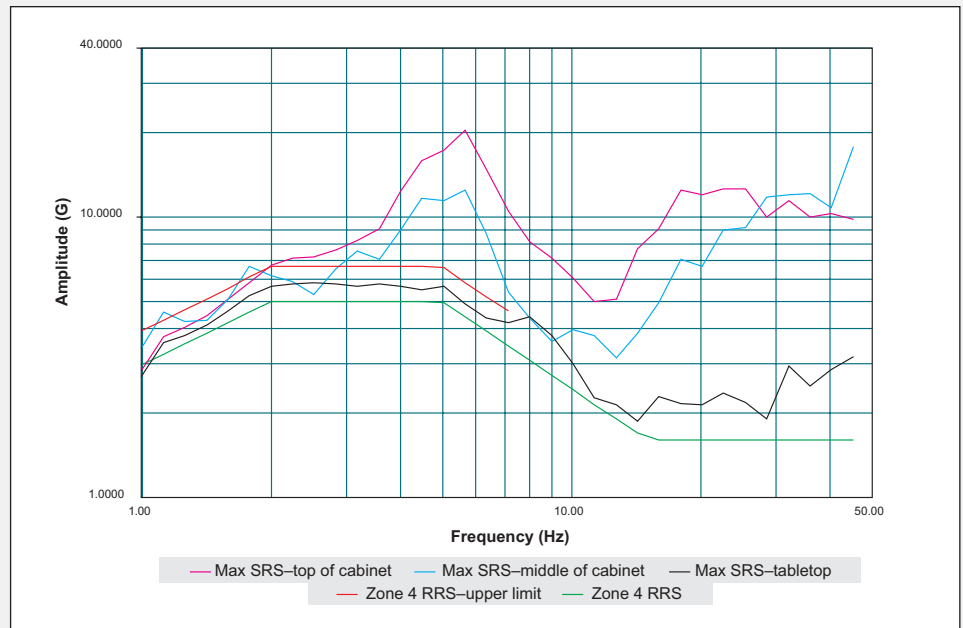
Figure 6 – SRS of the X-axis (side-to-side) for the zone 4 earthquake profile during system-level testing
